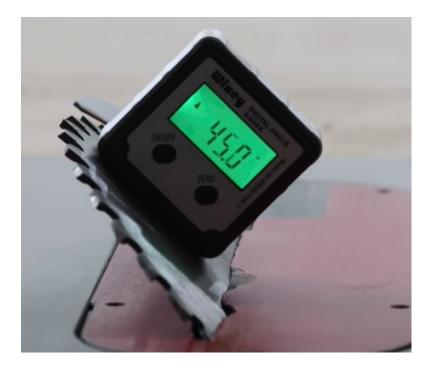
What this does, is guarantee that we will cut the bevel just a hair past 45 and that will result in our miter joints being closed at the top of the corner instead of the bottom when gluing up the entire box.
