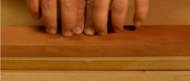
Now you can run them thru the router, do your pattern. The trick to this is that when you need to separate the pieces the painter's tape is gonna tear out and both pieces are not gonna suffer any damage from the CA glue.
