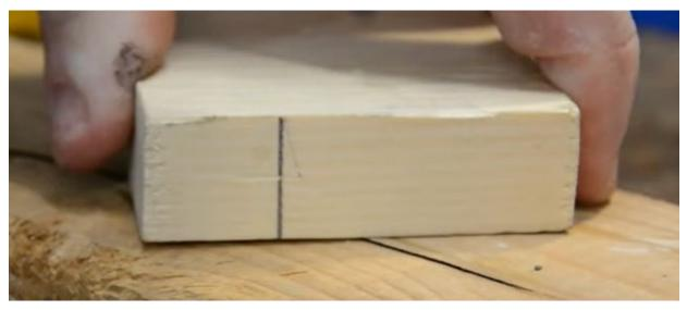
Use that line to calibrate one direction and the wood itself to calibrate the other direction as long as you keep them in line you'll get a straight hole every time.
