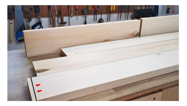
Then is just a matter of marking 2 diagonals using the square and making sure that the tips of those diagonals hit the perpendicular mark at the edge. Whenever those two lines meet is the center of the board.
