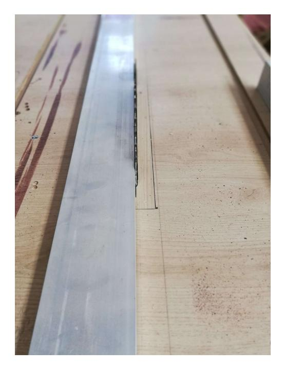
This line is exactly in line with my blade. Once I do one side I flip it over and I do the other side.
