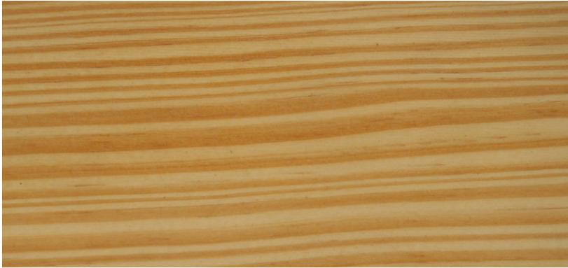
Sometimes confused with Ponderosa pine and western white and also known variously as yellow pine, Quebec pine and long leaf pine. This heavily-grained wood, with alternate streaks of cream and brown, is straight grained, coarse in texture with a high resin content. In former times this wood was used for chapel pews and furniture. (U.S.A.)
