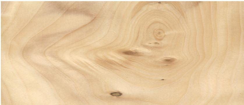
Known also as European white wood and European spruce, this pale-yellow to brown wood is straight grained and even textured with few knots and twists. It is used for interior framing, crates and pallets and in the making of musical instruments. If you want to try some low-cost woodwork, carving or joinery, then this is a good choice. (U.K. Europe, Russia)
