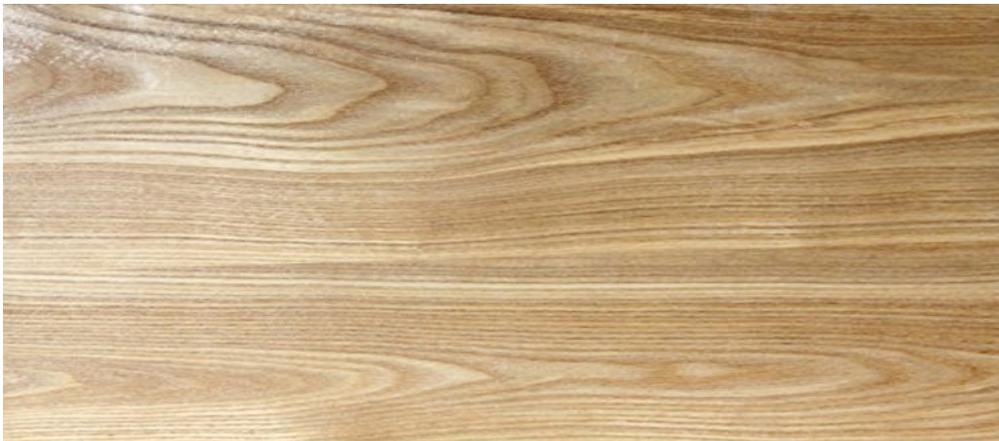
A long-grained, tough, grey to red-brown hardwood traditionally used for tool handles, chair legs, agricultural implements, baseball bats and items that needed to be steam bent. Although ash is extremely hard to work, the resultant pieces of woodwork are both attractive and long lasting. The European and American varieties have very similar characteristics. (U.K. Can. U.S.A.)
