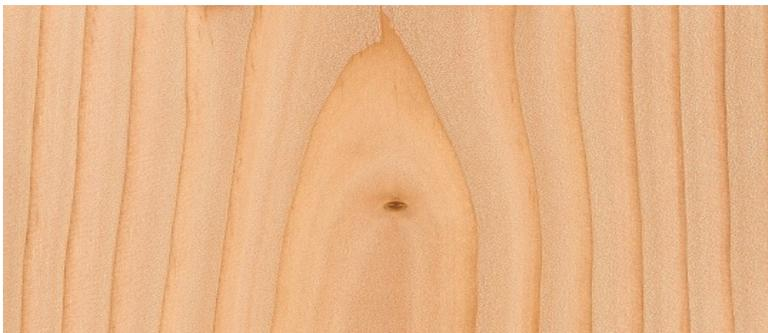
Known also as Columbian pine, red fir, Oregon pine and other names besides, it is a reddish-brown, straight-grained wood. In long lengths it is traditionally used for bridges, masts, pit props and residential construction. It is a good wood common interior joinery. Although difficult to work, it has an exciting grain pattern. (Canada, USA, UK, NZ, Australia)
