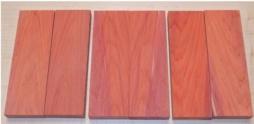
A soft, straight-grained wood with a fine, even texture, pencil cedar is used for making slats for lead pencils. It is also used for furniture, joinery, carpentry and for making cigar boxes. Due to its fragrant scent it is popular for linen chests and for interior furniture linings. (Canada, U.S.A.)
