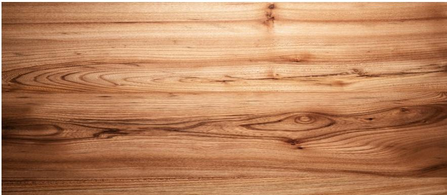
A light to reddish-brown wood with a straight grain and a slightly coarse texture. Traditionally used for ship building, wheel hubs and for agricultural implements. A good wood where you want a mix of lengths, strength and good bending qualities. (Canada, USA, Europe, N. Africa, India, China)
