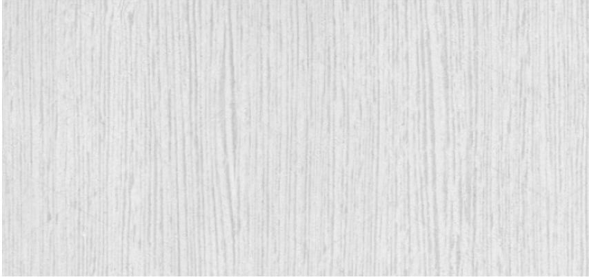
This is a creamy-white wood with a grey tint and a shallowly interlocked grain that works easily with either hand or machine tools. Pterygota is used for furniture fitments, joinery and carpentry, boxes, crates and pallets. It is also sliced for decorative veneers, that need careful handling as they are rather brittle. (Africa)
