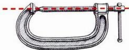
ABOVE: Clamp – it's vital that the screw and the ball-and-socket fixture are centered on the anvil.
