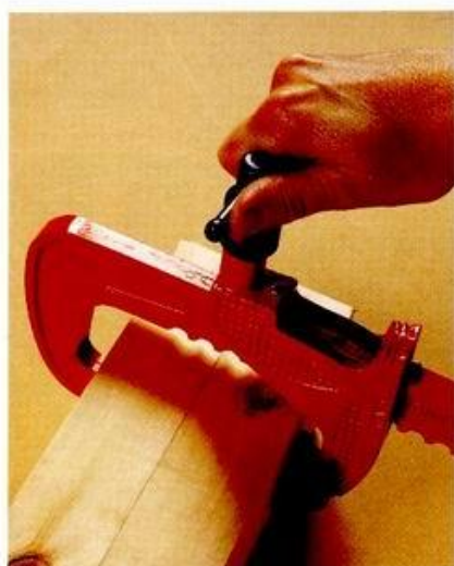
ABOVE: This particular clamp can be tightened up without any twist-damage action.
