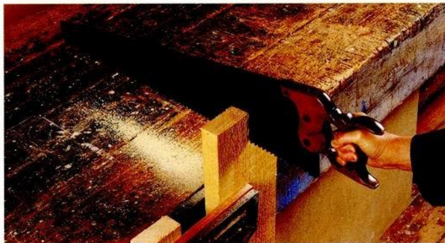
ABOVE: Ripping in a vise – let the weight of the saw do the work.
