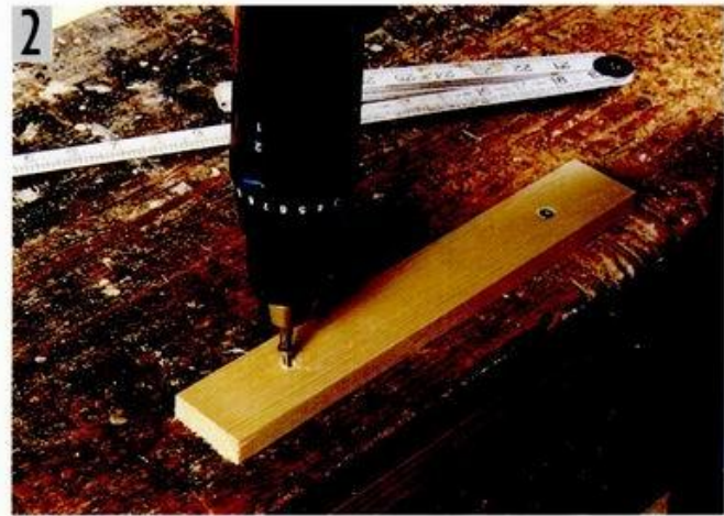
ABOVE: Home-made bench stop – two wedge type.
