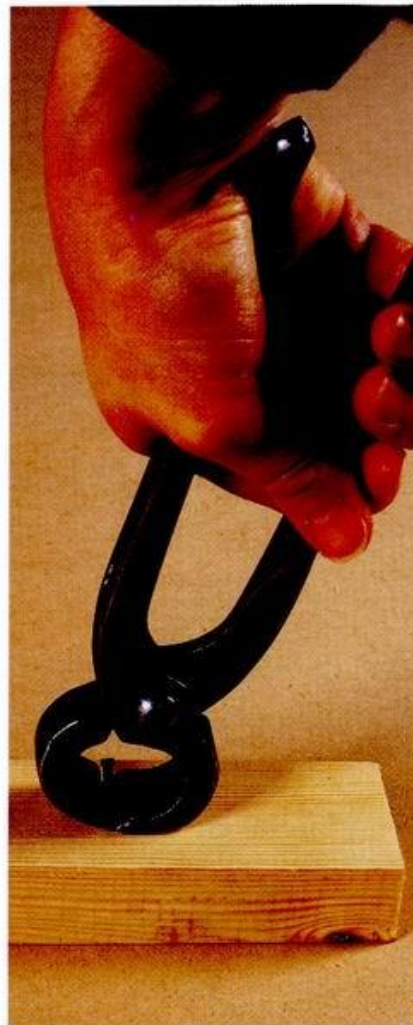
ABOVE: Grip the nail so the rounded jaws of the pincers are in contact with the workpiece.
