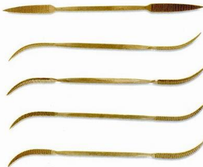
ABOVE: Riffler files, with shaped blades and rasp teeth – good for cleaning out difficult-to-reach spots.
