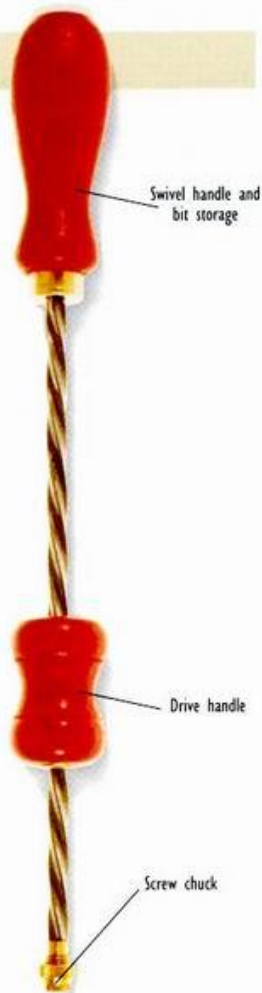
ABOVE: Archimedean drill, also called a fret drill, is used for boring small-diameter holes in thin-section wood.
