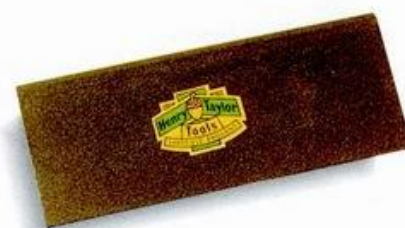
ABOVE: Shaped oil stone – used for sharpening woodcarving gouges.
