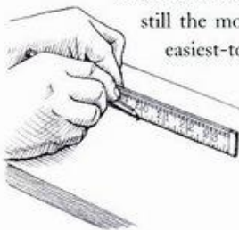
LEFT: The traditional boxwood rule is still a top quality tool. Place rule on edge for accurate markings.
