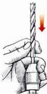
ABOVE: Putting the bit in the chuck.
