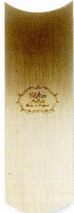
ABOVE: Scrapers are very useful for removing patches of rough grain in an otherwise smooth surface.
