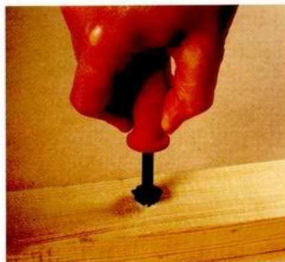
ABOVE: Give the hand countersink several quick swivel-turns.
