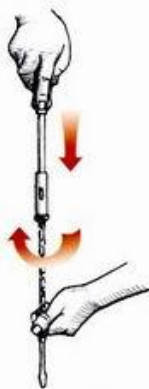
ABOVE: The Yankee-type screwdriver – with its chuck and selection of bits – is a great all-round tool.
