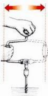
ABOVE: The sweep of the brace.
