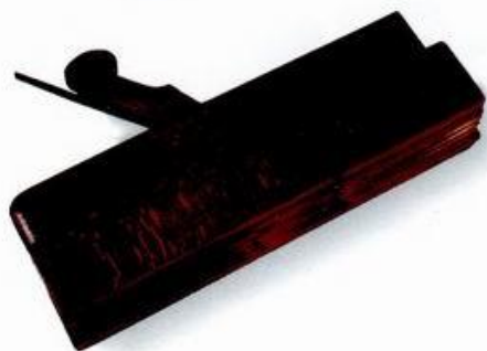
RIGHT: Triple-reed – a good quality plane with a fully-boxed sole.
