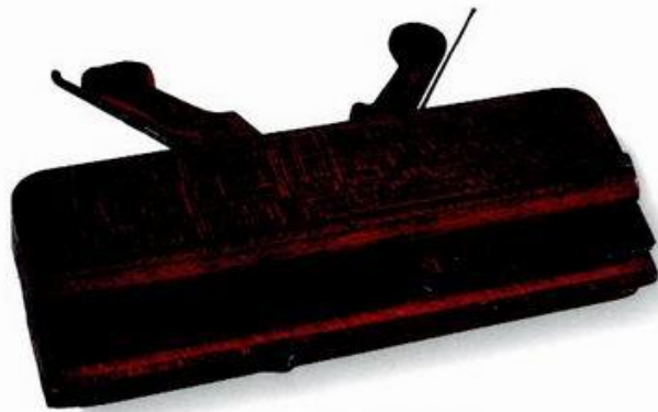
ABOVE: A 2-in-1 tongue and groove molding plane.
