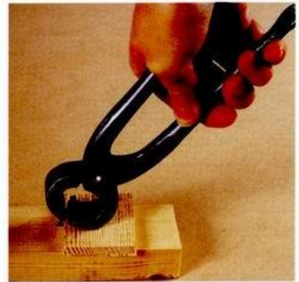
ABOVE: Lever the pincers down and over so the rounded jaws act as a fulcrum.
