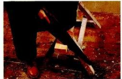
ABOVE: Raise the saw handle when the cut is under way.
