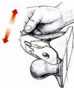
ABOVE: Move the lateral lever left or right to set the iron square in the mouth.
