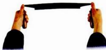
ABOVE: For full and safer control, always hold the drawknife with two hands.
