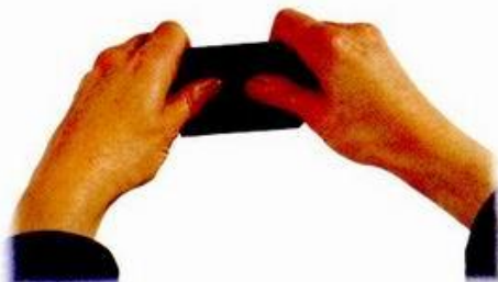
ABOVE: Bow the scraper with your thumb until it begins to “feel and bite.”
