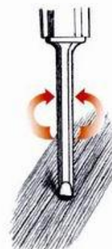
Thin blade used for picking out patterns and for marking
