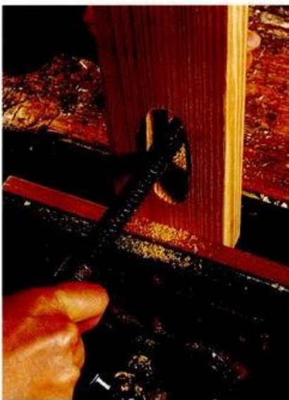
LEFT: Though the tube surform is a great tool for cleaning out curve-side pierced holes, you do have to be careful not to run directly into end grain.
