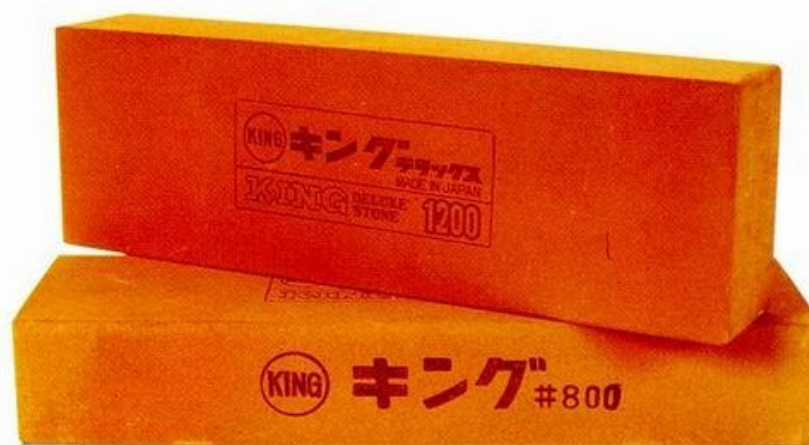
ABOVE: Japanese waterstones – single grit for general sharpening.
