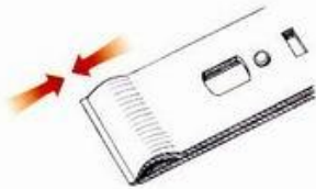
ABOVE: Setting the irons for rough work.
