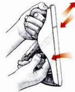
ABOVE: Adjust the depth of the cut by advancing or retracting the blade.
