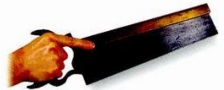
ABOVE: The handle of the dovetail saw is designed for maximum comfort. The notch at the top of the handle enables the woodworker to point and hook his index finger for optimum control.
