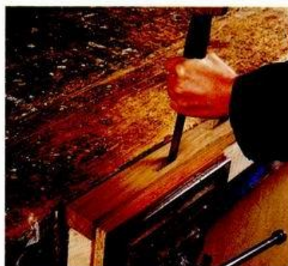
ABOVE: The block of waste under the workpiece takes the brunt of the blows.
