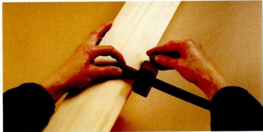
ABOVE: Spike the pin on the mark, slide the fence against the edge and tighten the screw.
