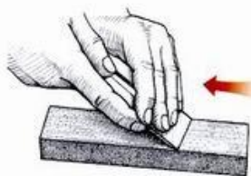
ABOVE: Honing the cutting edge.
