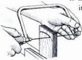
ABOVE: Holding and using the coping saw.
