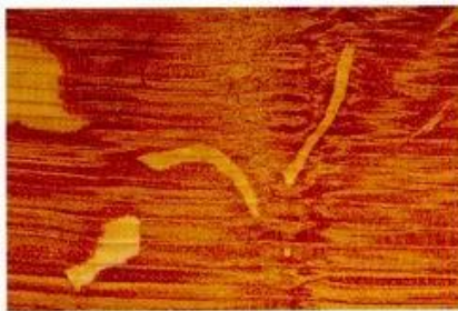
ABOVE: Quartersawn oak with characteristic medullary ray figure – strong and decorative.
