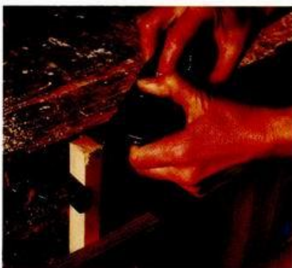
ABOVE: This set-up ensures that the damage occurs on the waster, rather than the workpiece.
